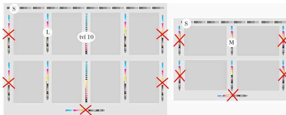
FIGURE 8 Positioning options for GrayCon versions on sheets or web cut-offs with long or short grain pages
